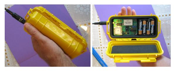
The Micro-Trak AIO features an SMA for the antenna connection so an adapter will probably be necessary for use with a higher-gain antenna.
